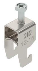
Clamp clip with U-foot, metal pressure trough with rounded edges to protect the cable. For vertical and horizontal mounting of 1 single cable on a C-profile rail. For slot width 18–22 mm. With 1-start screw thread on pressure trough, universal hexagonal screw head WAF10, with slot and cross recess. Suitable for mounting indoors and outdoors. We recommend the use of a counter-trough.
