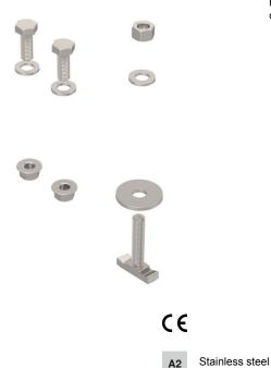
Screw set including hexagonal screws M12, hexagonal nuts with flange M12, hook-head bolt and washers. For the fastening of perforated straps, type LB FT, on rear supports on pre-assembled beams of PV open-field mounting systems.
