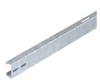
Support profile to mount photovoltaic modules on free-standing systems. Mounting of support profile on pre-mounted supports with KV FT cross-connectors. Mounting of the PV modules on the support profile with end and/or connection clamps. Connection of multiple support profiles with LV FT straight connectors and KV FT cross-connectors, screw-on.
