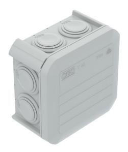
Junction box for the connection of cables indoors and in protected outdoor areas. Square design with plug-in seals to the sides and knock-out entries in the bottom. Suitable for wall and ceiling mounting and on mounting panels. With the option to fasten inside. With fixed clamping cover. Made from halogen-free, UV-resi-
