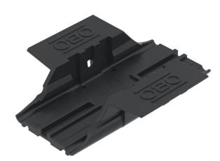
Adapter for TP 45 support profile, for mounting on UniBase universal stand. Toolless mounting through snapping. With side holes for optional screwing. Toolless mounting and dismantling of the support profile possible. With non-slip support surface.
